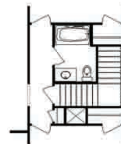
Partial Floor Plan with Basement Stairs
